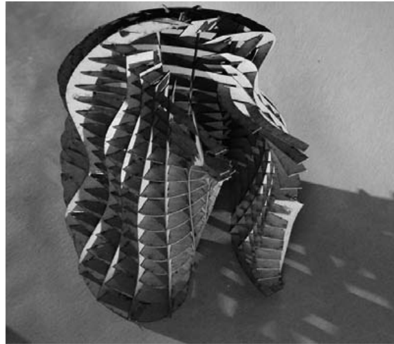
Fig. 1 the result of the application of the plug-in on a free form surface; the surface is transformed to a bilateral network of connected ribs. (Sass, Michaud, Griffith)
