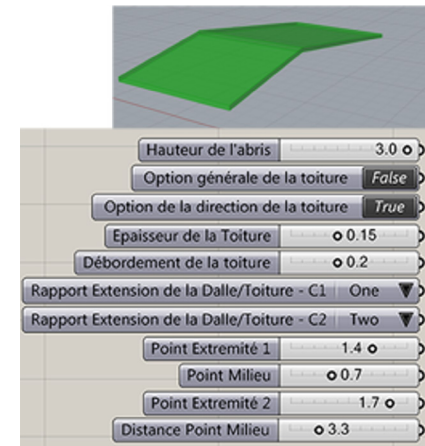
Figure 5 Roof generation process and parameters
