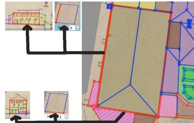
Figure 7: Relations between the edge of the ground polygon with their corresponding facade.
