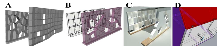
Figure 4. Box density optimization (quad/voronoi). A, 60/38. B, 24/30. C, 24/18. D, Assembly detail on mitre joints. Items are put together by using fasteners and bolts.
