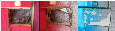
Fig. 7. Detail of a small and deep courtyard: on the left, the real scale model; in the middle, 123Dcatch finds an average round geometry; on the right, the scan leaves holes instead of proposing a fake geometry.
