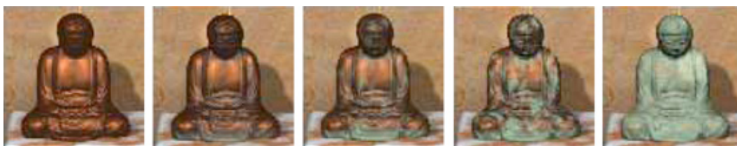
Figure 15: weathering sequence tested on a copper sculpture
