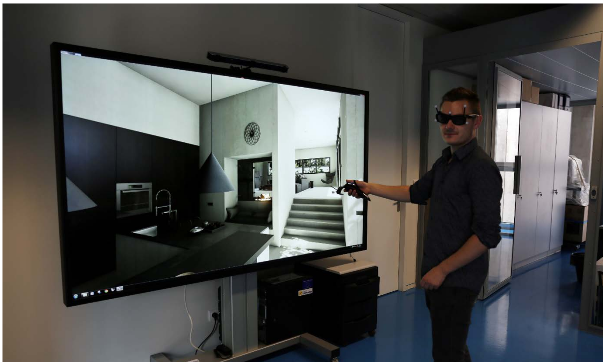
Figure 9. Wall system – motion tracking cameras, 4k screen, Senso, 3d glasses with some optical tracking targets.
