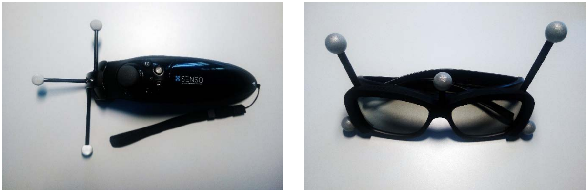
Figure 8. Senso and Glasses optical tracking targets.
