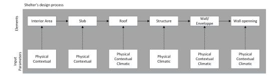
Figure 1 Shelter's design process
