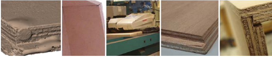
Figure 7. A, 3d scanned image of an unsuccessful rabbet. B, Mitre joint. Angles not coupling well after cutting. C, Manual correction of mitres and rabbets. D, An item containing both a successful mitre and rabbet. E, Correct coupling with rabbet joints.
