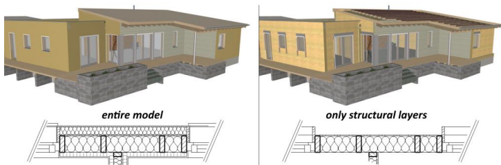
Figure 9. Selection of information in ArchiCAD before the IFC export
